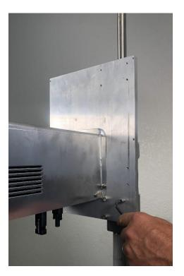
This next step is very important. We will need to make sure the piston is in the correct position. To do this, grab the portion of the 13" rod extension that is sticking out of the top of the unit and pull up. The ideal location for the joint between the standard pump rod and the 13" extension is in the middle of the clevis, as shown in the photo to the right, circled in red. If your rod to pipe ratio is correct, you should need to lift the rod up to get it into the position explained above.
