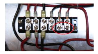
If you are planning to integrate a pressure switch you can use a standard pressure switch. When using DC voltage, you can simply jumper the two middle terminals and add your supply wire to one of the outer terminals and the return wire to the other outer terminal.
