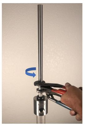
Add the 13" Rod Extension to the top of the existing pump rod. As mentioned above, these are reverse threads so you will go counterclockwise to tighten. Use the two channel locks to tighten.
