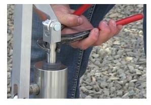
Remove the lever arm bracket and lever (they should still be connected) from the 3/4" stainless rod. These are reverse threads, the direction you screw is the opposite of normal -- turn clockwise to remove, rather than the normal counterclockwise.
