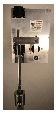
Lower the assembly onto the pump head so that the pump rod and extension are inserted through three (3) openings. As the unit is lowered down, the rods move through the below pieces, in order.
