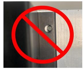
The adjustment for this requires that you loosen the four (4) ¼-20x3/4 SS cap screws holding the unit to the pump head. Lift up on the bottom right corner of the mounting plate slightly and tighten the four mounting bolts. Check the alignment between the holes in the top linear bearing and the mounting plate again. Make as many adjustments as necessary to get the holes lined up like the image to the right.
